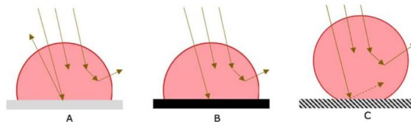
**Figure 1.** Visualization if (A,B) the transmitted light influences the reflected light for the different colored backgrounds, and if not (C). The striped surface for C indicates a similar result for both background colors.
