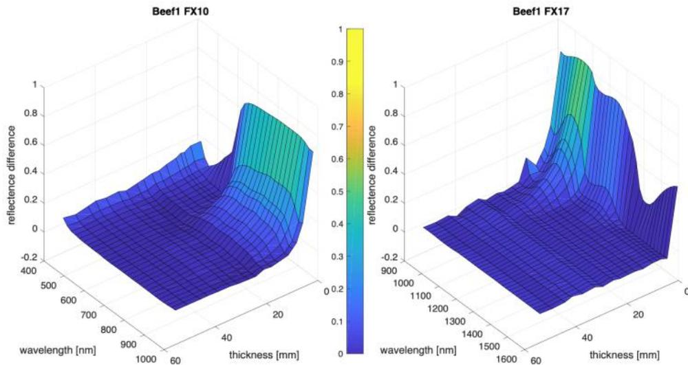
Figure 2. Three-dimensional plots of thickness, wavelength, and reflectance difference for beef tomato sample 1.
