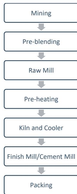
**Figure 1.** Steps of cement production by PT X.
