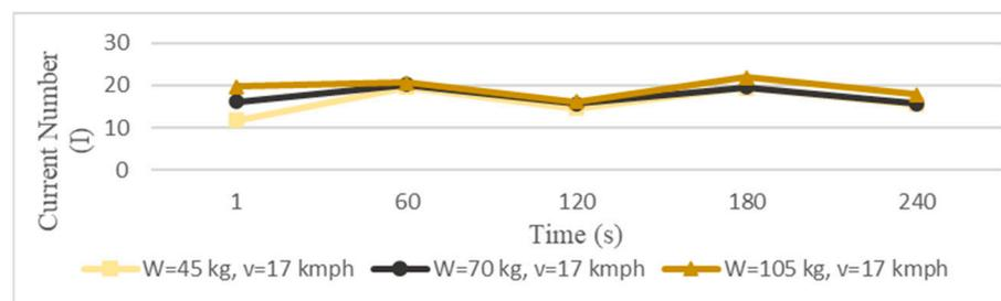
**Figure 8.** The current number for various weights at 17 km/h.
