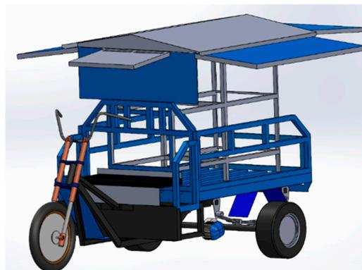
**Figure 1.** Design of three-wheeled electric vehicle.
