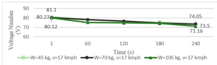
**Figure 6.** Voltage for various weights at 17 km/h.
