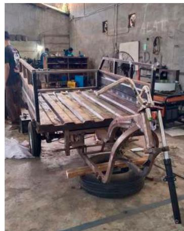
**Figure 3.** Mechanical components assembly after welding process.
