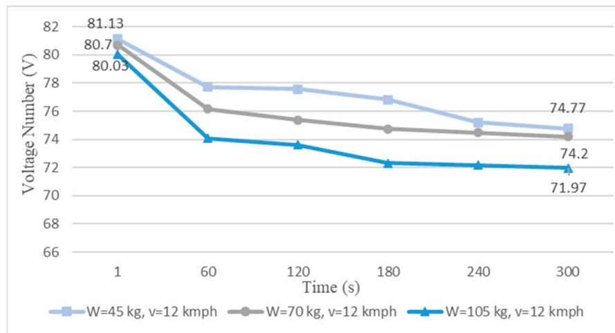
**Figure 5.** Voltage for various weights at 12 km/h.
