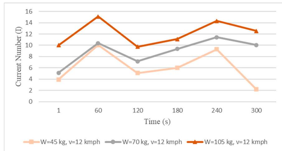
**Figure 7.** Current number for various weights at 12 km/h.
