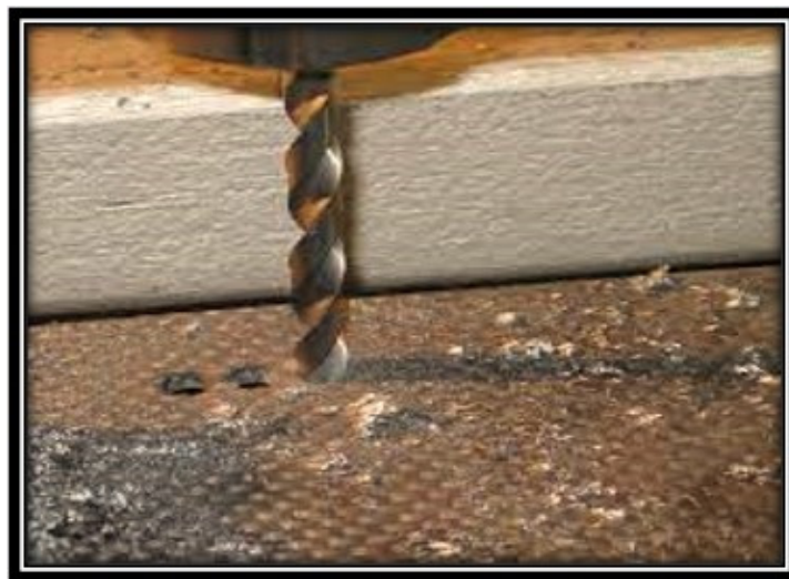
Figure 1. Depicts the photographic image of the drilling of kenaf/PLA composite materials.
