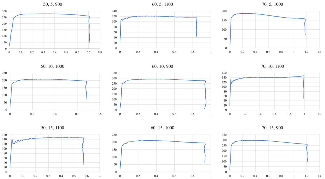
Figure 1. Stress–strain curves for the L9 array.
