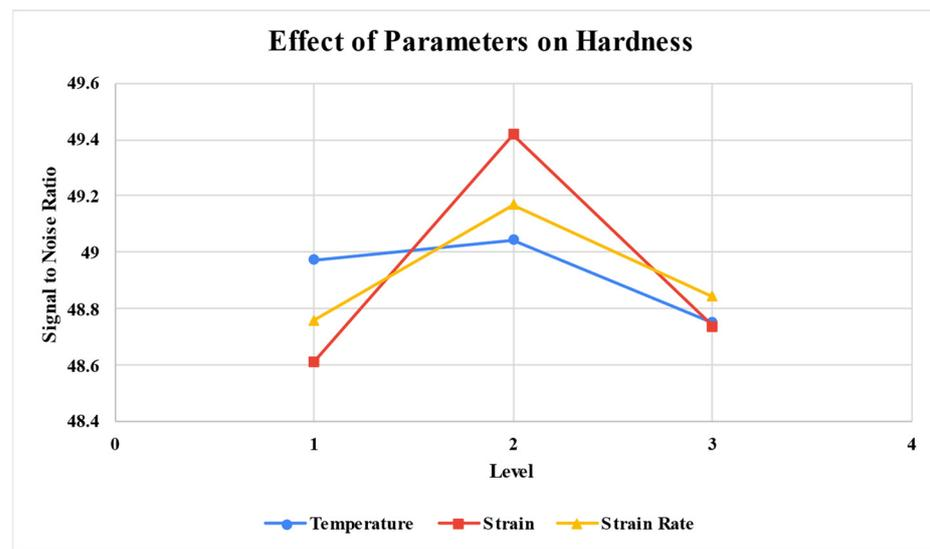
**Figure 3.** Effect of different parameters on hardness.
