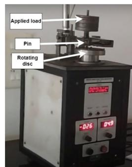
**Figure 3.** Wear test machine used in this research.
