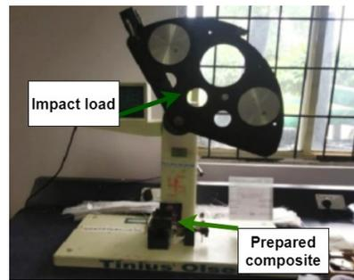
**Figure 2.** Impact test specimen.
