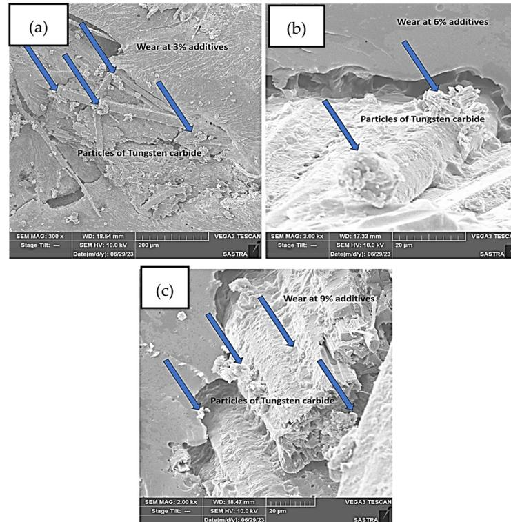
**Figure 7.** SEM analysis of the prepared composites of varying composition of WC (a) 3% WC reinforcement (b) 6% WC reinforcement (c) 9% WC reinforcement.
