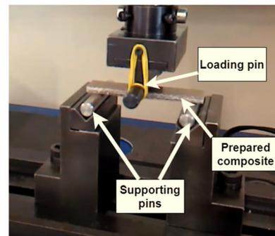
Figure 1. Flexural test.
