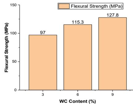
**Figure 4.** Flexural strength of the composite.
