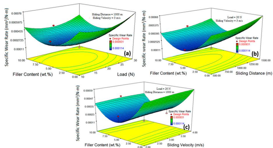
**Figure 1.** Contour plots of (a) Filler—load influence on SWR, (b) Filler—sliding distance influence on SWR, and (c) Filler—sliding velocity influence on SWR [2].
