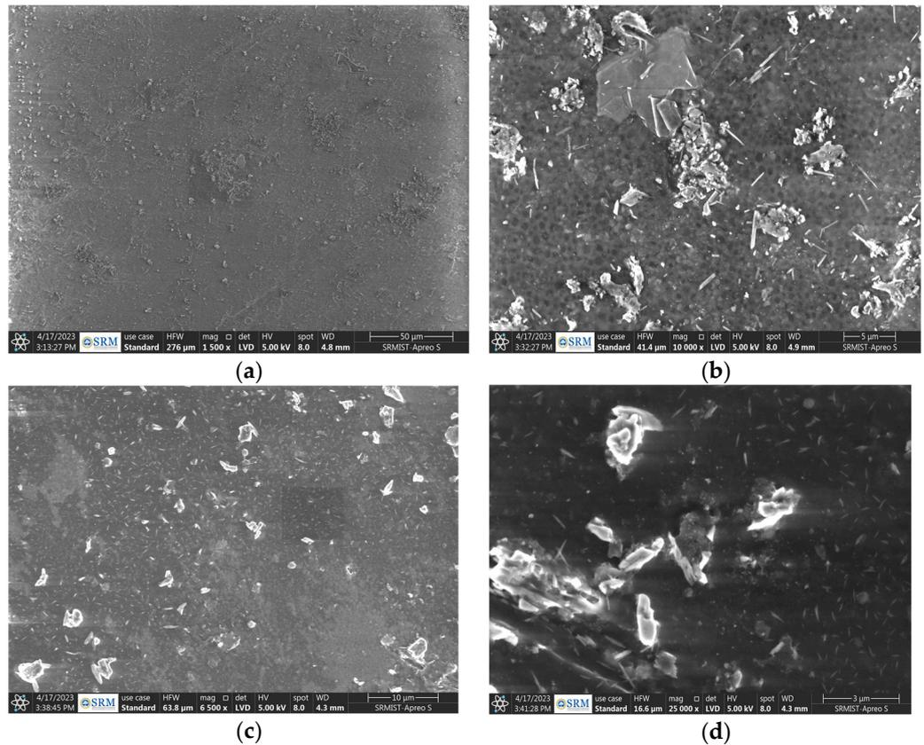
Figure 2. SEM images of (a) cassava bioplastic with 500×, (b) cassava bioplastic with 10,000×, (c) sweet potato bioplastic with 500×, (d) sweet potato bioplastic with 25,000×.
