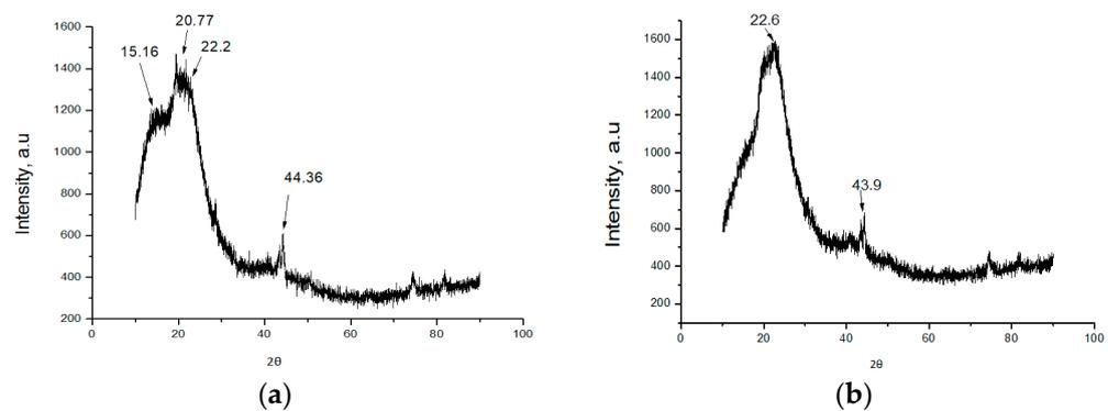
**Figure 3.** X-ray diffraction pattern of (a) sweet-potato-derived bioplastic; (b) cassava-derived bioplastic.
