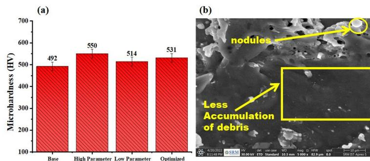
Figure 3. (a) Microhardness; (b) SEM graph of optimal WEDM parameters.
