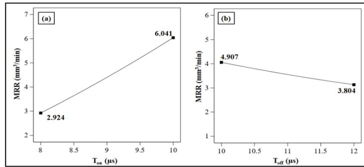
Figure 1. (a,b) Parametric effect of surface plots on the MRR.
