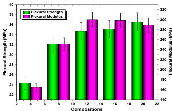
**Figure 2.** Flexural strength and modulus of NaOH-treated banana/CEP-based hybrid composites with different composition of filler.
