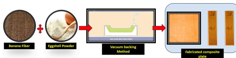
**Figure 1.** Schematic representation of composite fabrication process.
