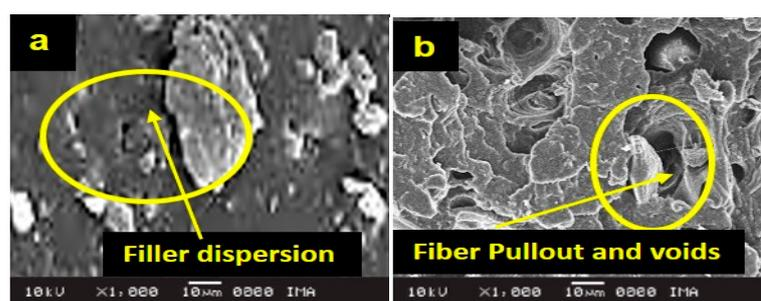
**Figure 5.** SEM image of banana-based hybrid epoxy composites (a) 4 wt.% of ESP filler; (b) 16 wt.% of ESP filler after flexural testing.
