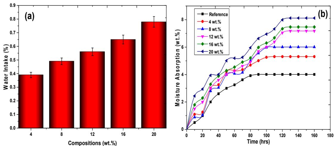
**Figure 4.** (a) Overall absorption rate; (b) water absorption potential of composite at different hrs.
