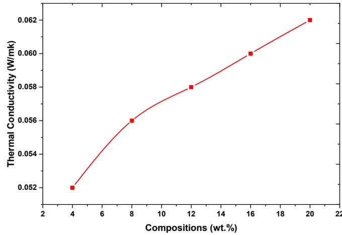
**Figure 3.** Thermal conductivity of NaOH-treated banana/CEP-based hybrid composites with different compositions of filler.
