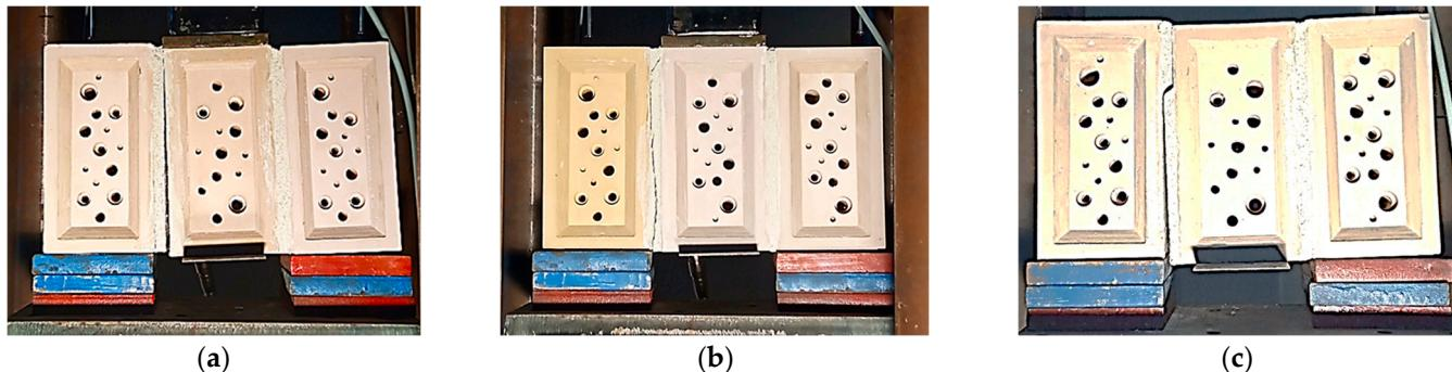
**Figure 5.** Failure modes of brick triplet subjected to shear testing for types (a) A1, (b) B, and (c) A2.
