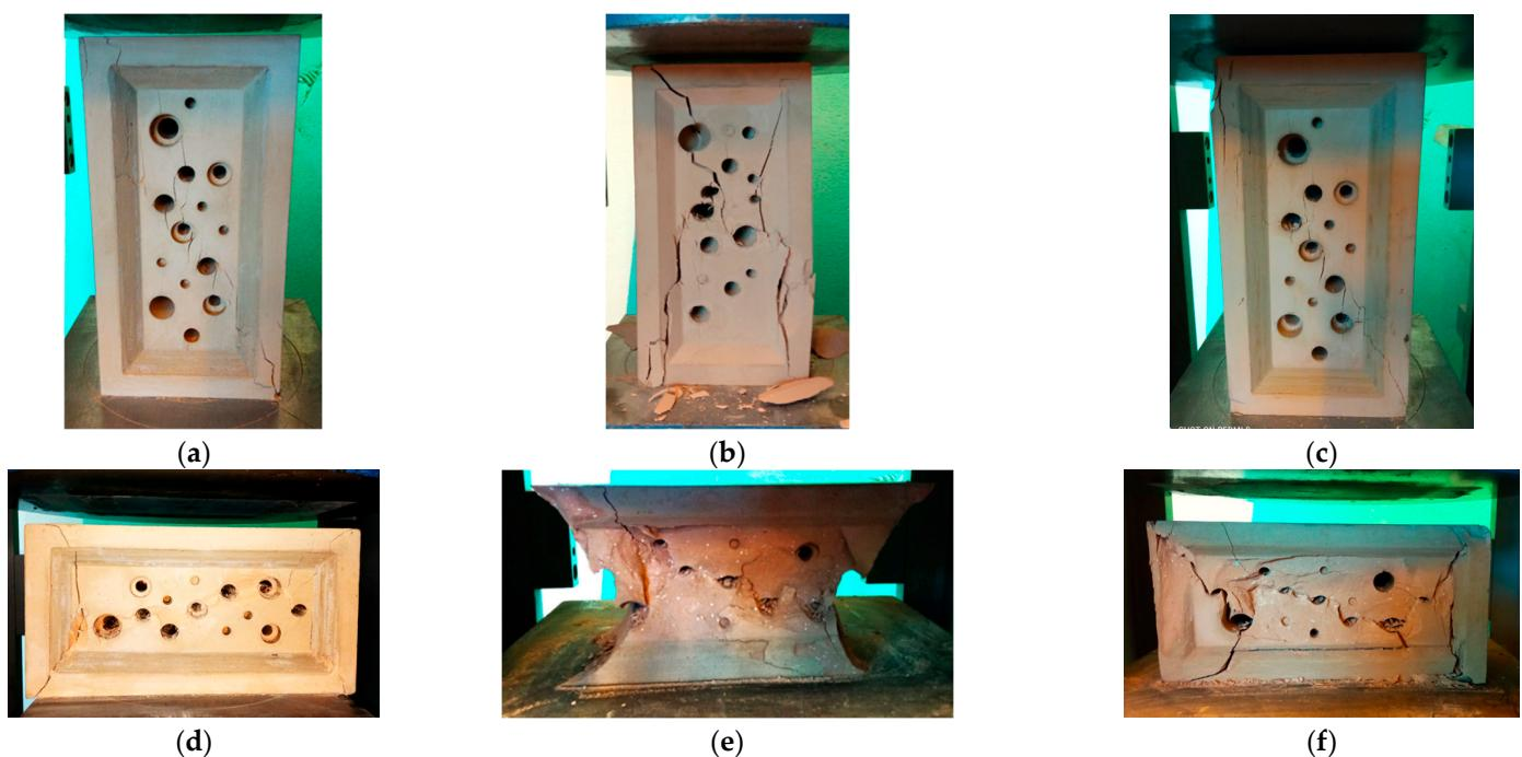
**Figure 3.** Failure modes of characteristic bee bricks with the loading direction (a–c) perpendicular to the bed joints and (d–f) parallel to the bed joints.
