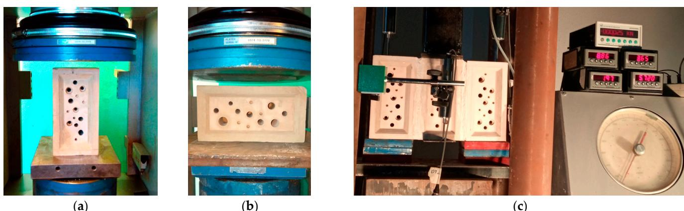
**Figure 2.** Experimental test setup of (a) compression test of solid brick with the loading direction perpendicular to bed joints; (b) compression test of solid brick with the loading direction parallel to bed joints; (c) direct shear test of brick triplet with Kerakoll binding mortar.
