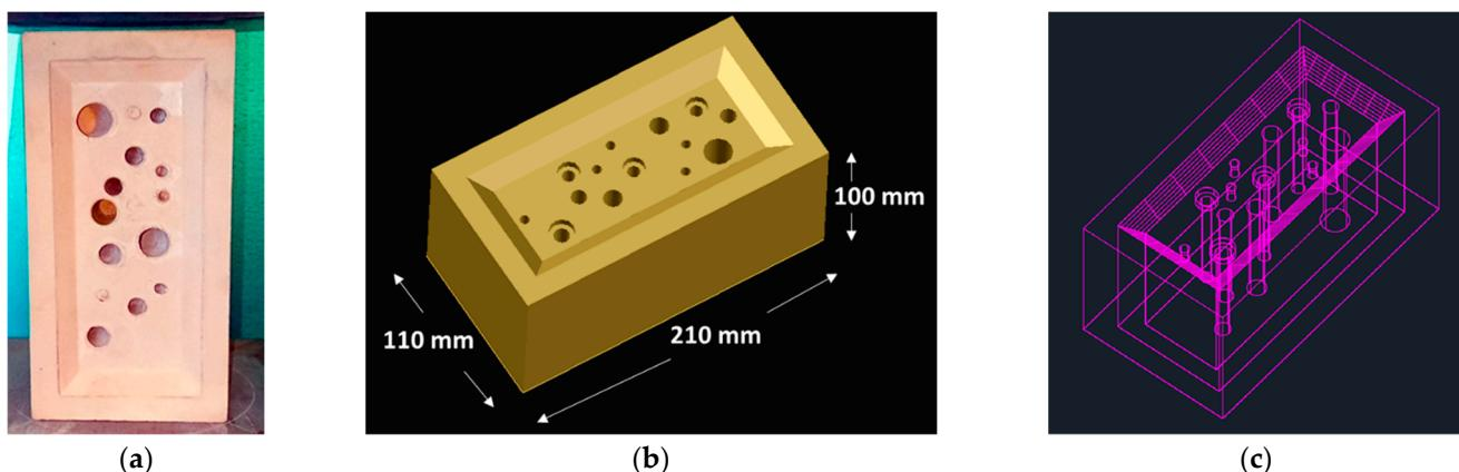
**Figure 1.** Bee brick (a) front view; (b) AutoCAD 3D-designed; (c) solid 3D-designed.
