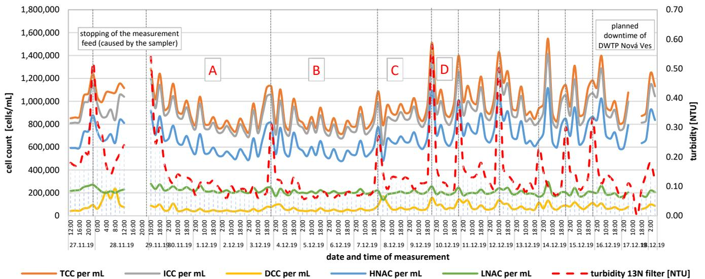
Figure 5. The 2nd stage of measurement from 27 November to 18 December 2019: FCM and turbidity (detailed A–D cycles are in Figure 6).
