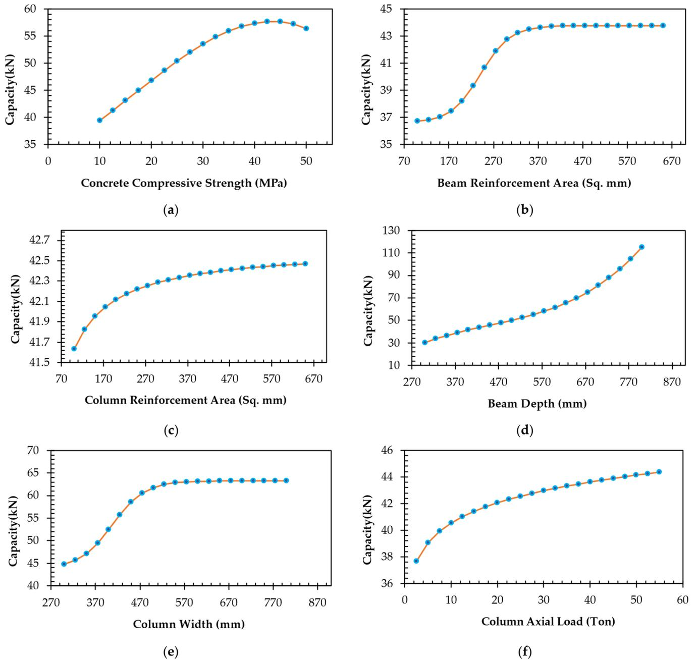
**Figure 4.** Parametric study: (a) capacity vs.  $f'_c$ ; (b) capacity vs.  $A_b$ ; (c) capacity vs.  $A_c$ ; (d) capacity vs.  $D$ ; (e) capacity vs.  $B$ ; (f) capacity vs.  $P$ .
