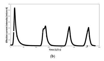
**Figure 4.** Change in the effective current intensity as a result of the turning on/off of the incandescent light bulb (a) and behaviour of the NTC material under four successive thermal pulses (b).
