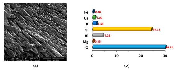
**Figure 2.** SEM-micrograph showing the lamellar texture of the clinoptilolite mineral (**a**) and its chemical composition obtained via EDS-analysis (**b**).
