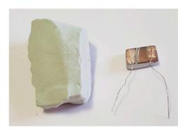
**Figure 1.** Fabricated NTC thermistor and starting clinoptilolite mineral.
