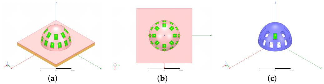
**Figure 1.** Measurement configuration: in (a,b) two views with  $N = 20$  slot antennas are deployed over a hemispherical cup which hosts the breast under test, in (c) picture of hemispherical cup in absence of the breast.
