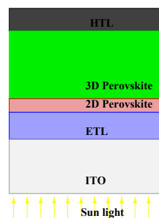
Figure 1. Device architecture of 2D/3D perovskite solar cell.
