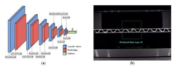
**Figure 3.** (a) The structure of the convolutional neural network applied in this work and (b) the real-time vision system.
