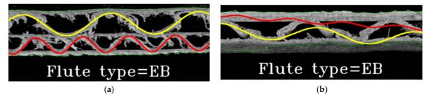
**Figure 5.** Examples of corrugated board samples with (a) jagged edges and cellulose fibers and (b) bent liners.
