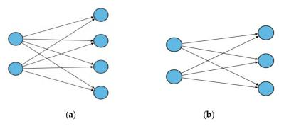
**Figure 2.** Structures of the feedforward artificial neural networks for the classification of corrugated board type for **(a)** double (5-ply)- or **(b)** single (3-ply)-walled corrugated boards.
