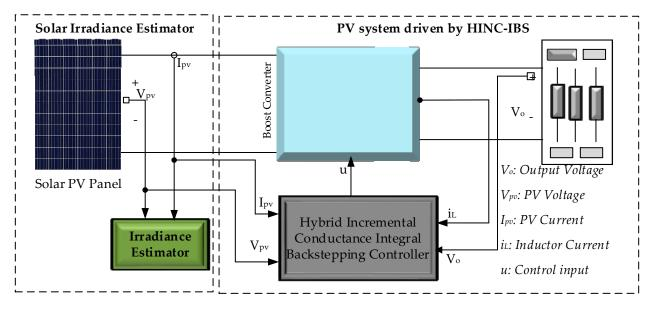
Figure 1. Block Diagram of the proposed system.
