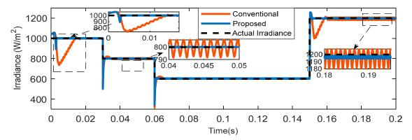
Figure 3. Simulation results of the estimators under fast-changing irradiance and temperatures.
