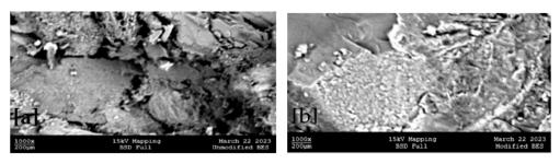
Figure 5. SEM morphology of (a) unmodified BES and (b) CCP-POFR-modified BES.
