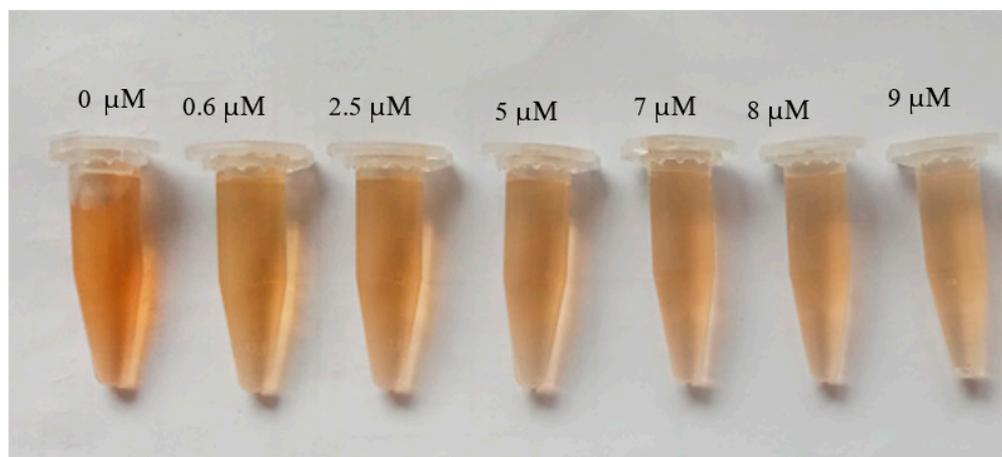
**Figure 4.** Color changes with different concentrations of mercury.
