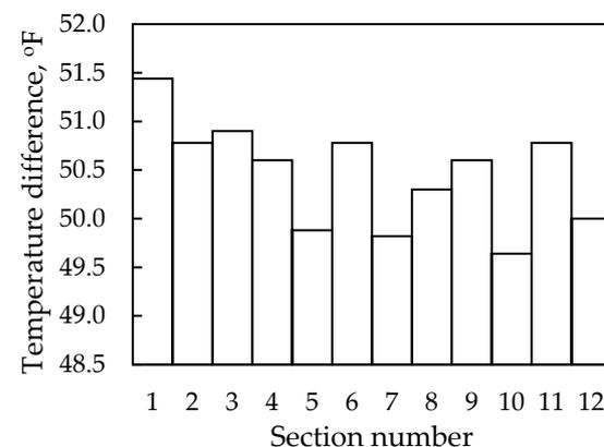
**Figure 3.** Temperature area distribution across the cross-section of an evaporating cooling tower with an irrigation area of  $2600\text{ m}^2$ .
