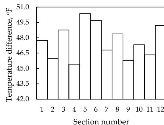
**Figure 2.** Temperature area distribution across the cross-section of an evaporating cooling tower with an irrigation area of  $1600\text{ m}^2$ .
