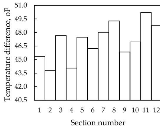
**Figure 4.** Temperature area distribution across the cross-section of an evaporating cooling tower with an irrigation area of 3200 m<sup>2</sup>.
