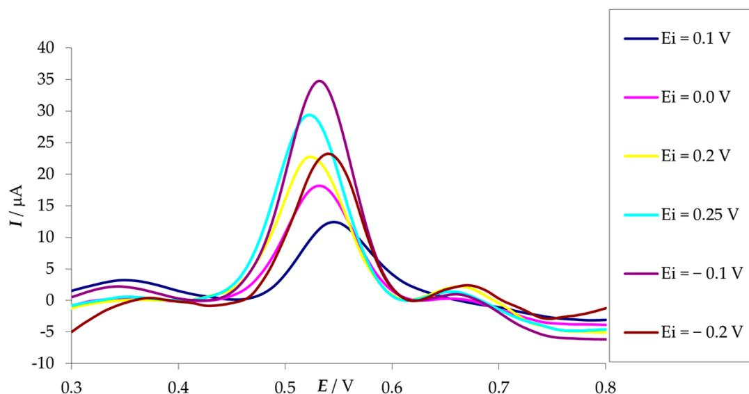
**Figure 3.** Comparison of voltammograms obtained during Stage II of the procedure for different values of  $E_i$  used in Stage I.
