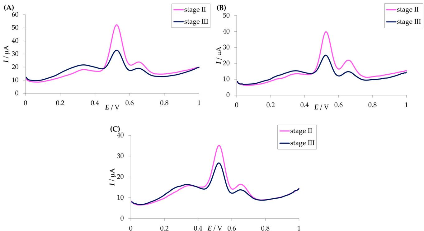
**Figure 4.** SWV voltammograms obtained during Stages II and III, after immersing the electrode in solutions of metal cations: (A)  $\text{Ca}^{2+}$ , (B)  $\text{Mg}^{2+}$ , and (C)  $\text{Fe}^{3+}$  at a concentration of  $C = 1.0 \times 10^{-6} \text{ mol}\cdot\text{L}^{-1}$ .
