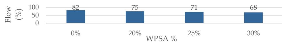
**Figure 1.** Flow/workability of 0, 20, 25, 30% WPSA mortar mix.
