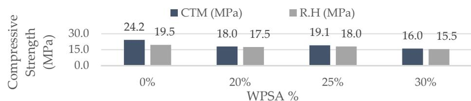
**Figure 2.** Compressive strength results (CTM and RH).
