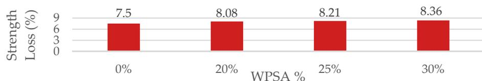
**Figure 5.** Loss of strength (%) in WPSA mortar samples.
