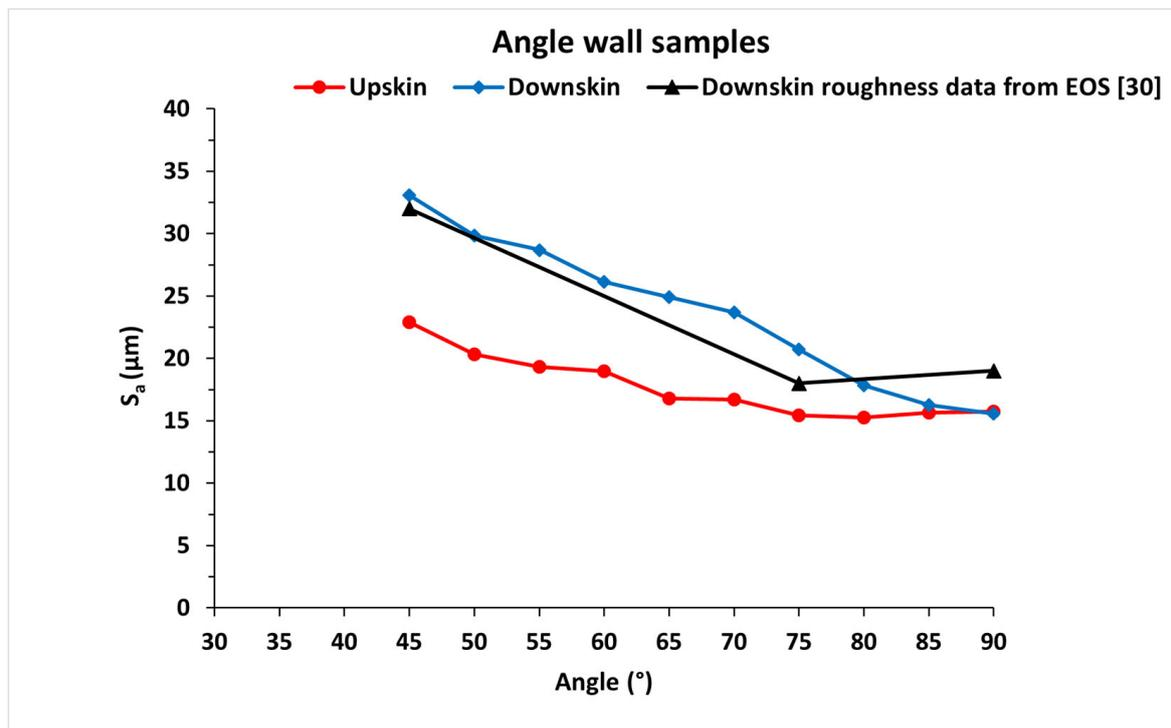
**Figure 5.** Influence of build angles on surface roughness of upskin and downskin surfaces [30].
