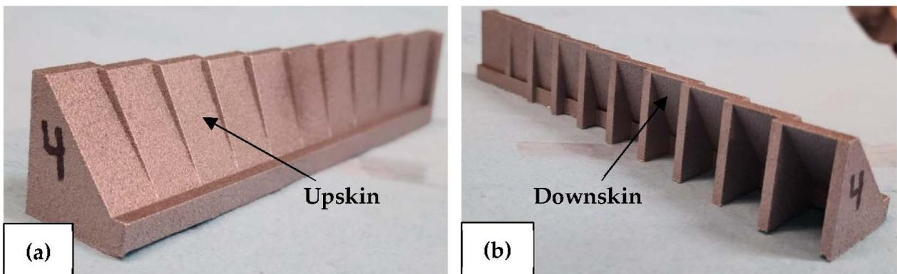
**Figure 3.** LPBF-fabricated angle walls showing (a) upskin and (b) downskin.
