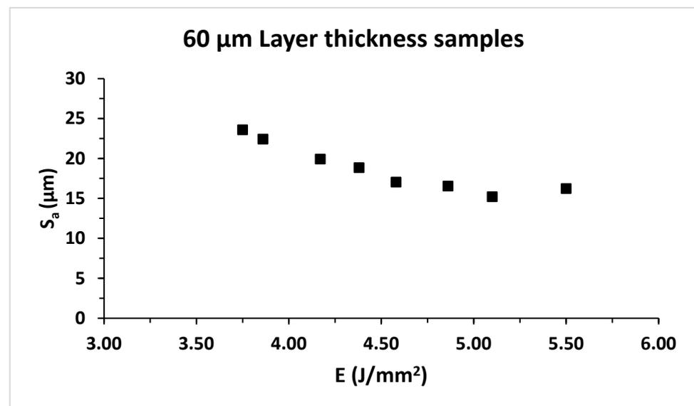
**Figure 4.** Variation of  $S_a$  with energy density (E) fabricated using 60  $\mu\text{m}$  layer thickness samples.
