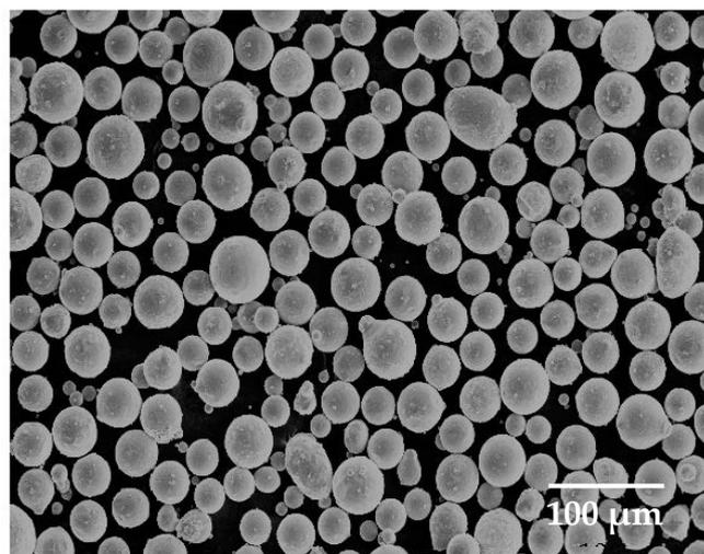
**Figure 1.** SEM micrographs of F357 powder.
