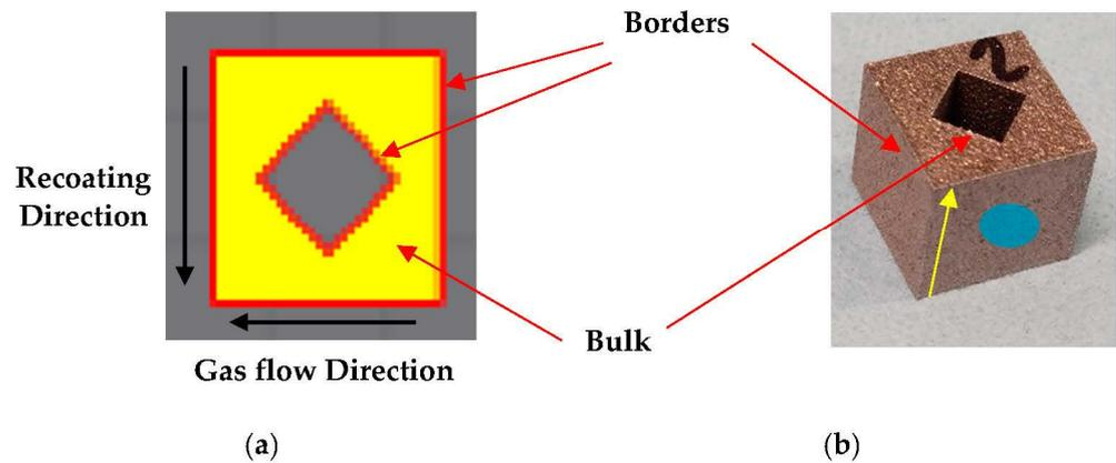
**Figure 2.** (a) Schematic showing borders of cube samples with diamond-shaped hole. The powder recoating and gas flow directions are also annotated. (b) LPBF-fabricated sample (yellow arrow shows the build direction, and blue marking depicts the side wall surface on which surface measurements were performed).
