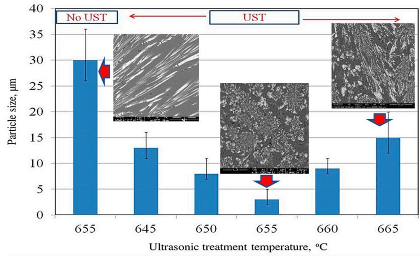
**Figure 5.** Average Al<sub>11</sub>Ce<sub>3</sub> particle size under different ultrasonic processing conditions [17] [edited-CCC permission].
