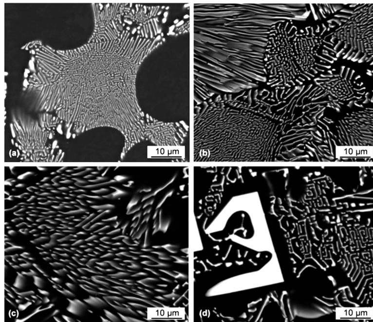
**Figure 2.** SEM micrographs emphasizing the shape and volume fraction of  $\text{Al}_{11}\text{Ce}_3$  in (a) Al-5Ce, (b) Al-10 Ce, (c) Al-15 Ce, and (d) Al-20 Ce alloys [18-Open access permission].
