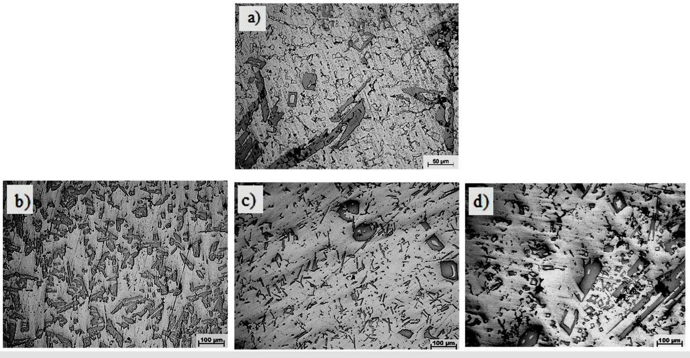
**Figure 4.** Optical micrographs comparing the intermetallic particle size of (a) solidified alloys without and with mechanical vibrations at (b) 655 °C, (c) 665 °C, and (d) 675 °C [22].
