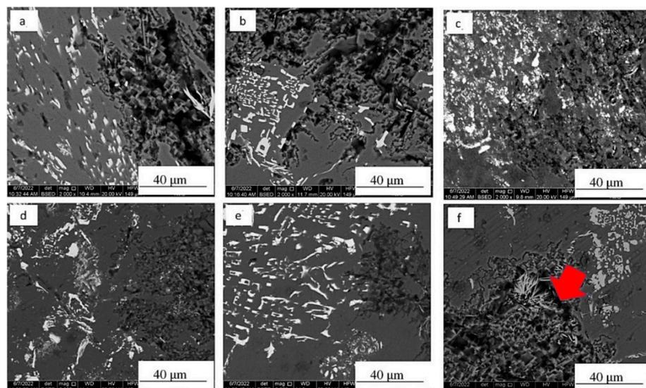
**Figure 6.** SEM micrographs of the corroded samples showing the influence of ultrasonic processing on the pitting susceptibility of Al-10 wt% Ce alloy at (a) 655 °C (untreated) and when ultrasonically treated at (b) 645, (c) 650, (d) 655, (e) 660, or (f) 665 °C. [30-CCC permission].
