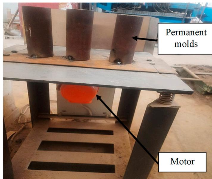
**Figure 3.** The settings of the permanent molds and the mechanical vibrators.
