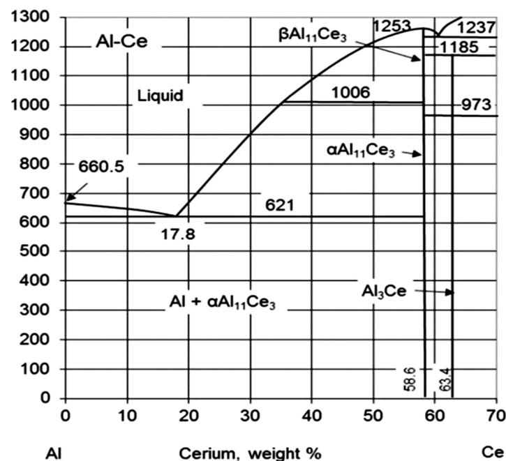
Figure 1. Al-rich Ce partial phase diagram [12], with permission 5626391072716 (copyright license number).
