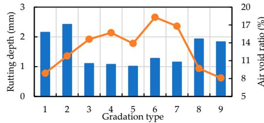
Figure 2. Results of the immersion rutting test.
