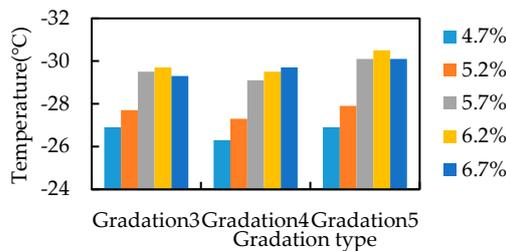
Figure 4. Results of TSRST test.
