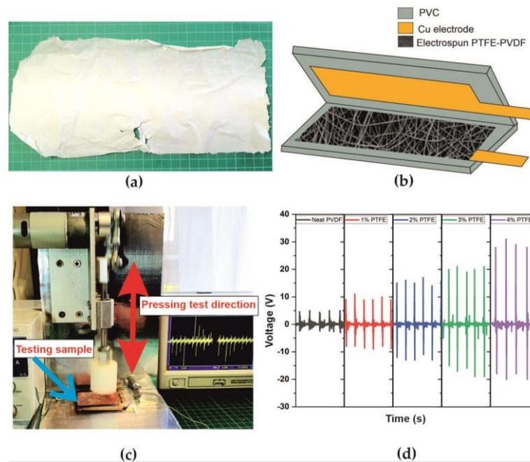
**Figure 1.** (a) PTFE/PVDF fibre mats after the electrospinning process of the 4%wt PTFE in the PVDF sample; (b) the schematic of the booked shape assembly for the testing cell PTFE/PVDF fibre sandwich with electrodes; (c) the compression test rig; (d) voltage output from constantly tapping the booked shape PTFE/PVDF fibre assembly at different PTFE concentrations of 0, 1, 2, 3, and 4%wt., respectively.
