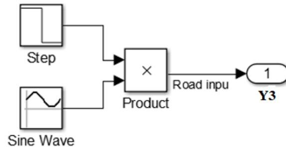
**Figure 6.** The bumpy road input’s Simulink model.
