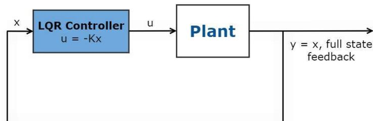
Figure 10. Schematic of the LQR controller.
