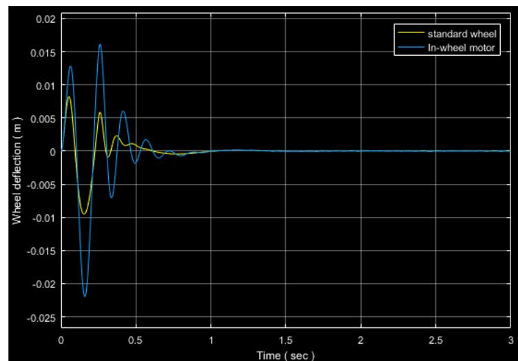
Figure 14. Wheel deflection with the bumpy road input.
