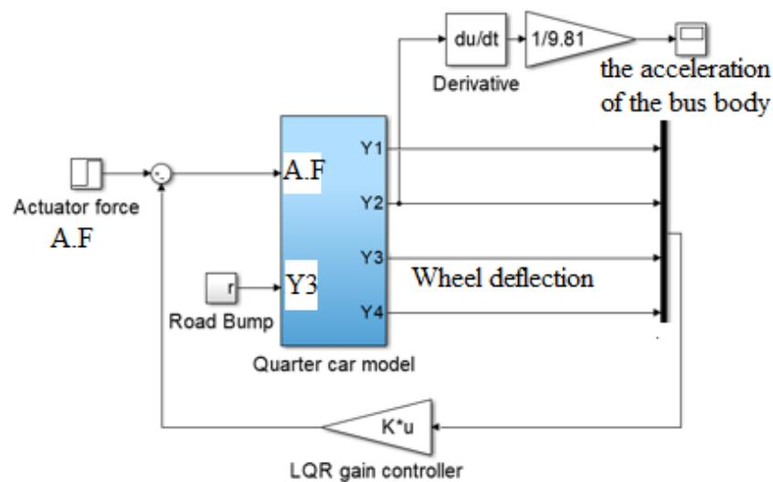
Figure 11. Active suspension system Simulink structure.
