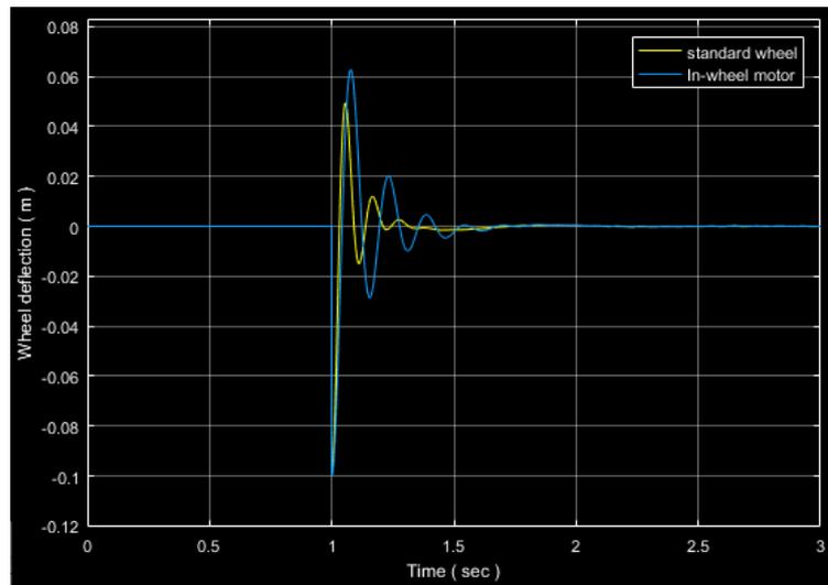
Figure 12. Wheel deflection with the step input.
