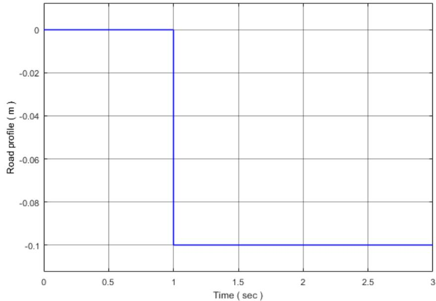
Figure 9. Unit step road signal.
