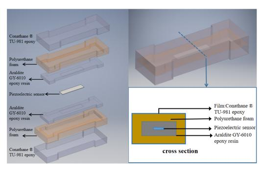
Figure 1. Configuration of the strain sensor.
