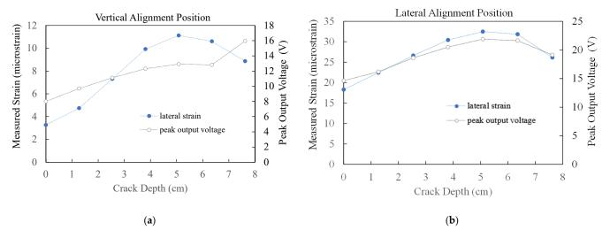
**Figure 4.** Measured lateral strain (along the x-axis) and peak piezoelectric-based sensor output in response to the depth of the bottom-up crack when the dynamic load moving velocity equals 25 km/h: (a) sensor is vertically aligned (along the y-axis); (b) sensor is laterally aligned (along the x-axis).
