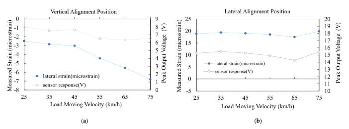
**Figure 3.** Measured lateral strain (along the x-axis) and peak piezoelectric-based sensor output in response to the dynamic load moving velocity when there is no bottom-up crack existing in the asphalt concrete pavement (crack depth = 0 cm): (a) sensor is vertically aligned (along the y-axis); (b) sensor is laterally aligned (along the x-axis).
