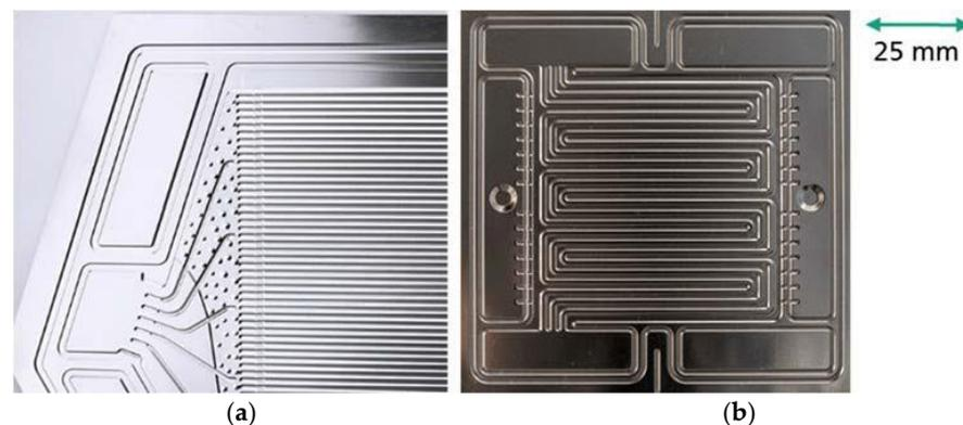
**Figure 6.** Bipolar plates produced by (a) active hydroforming, (b) passive hydroforming.
