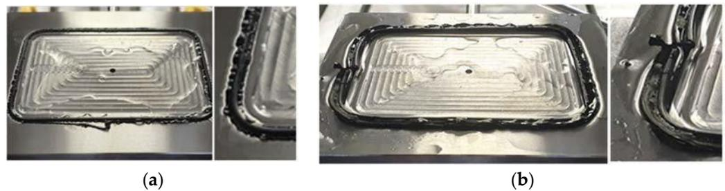
**Figure 7.** O-ring sealing-failure cases: (a) O-ring starts to flow and (b) O-ring seal failure at 200 MPa.
