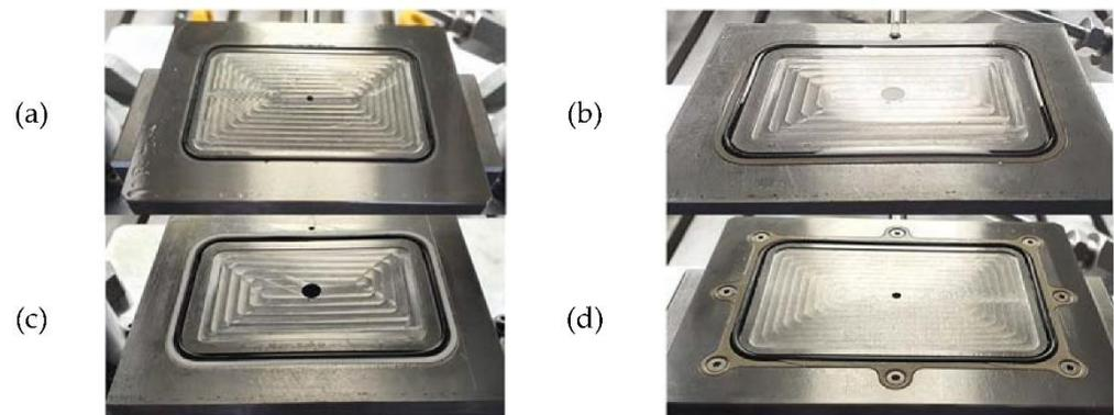
**Figure 5.** Filling plates with different sealing systems: (a) sealing with O-ring, (b) sealing with O-ring and milled one-piece support ring, (c) sealing with O-ring and 3D-printed one-piece support ring, (d) sealing with O-ring and milled multi-piece support ring.
