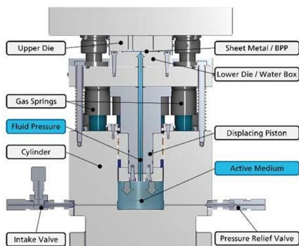
Figure 3. Cross section of a tool for passive hydroforming during pressure-build-up phase.
