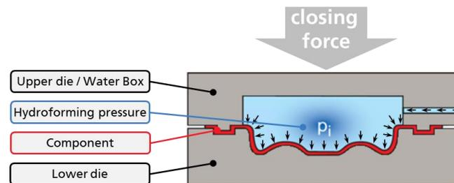
**Figure 1.** Process principle and components for active hydroforming of bipolar plates according to [3].
