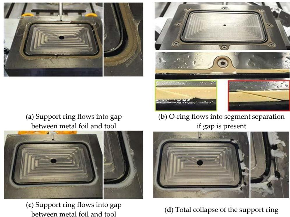
**Figure 8.** Sealing-failure cases (O-ring with support ring): (a) one-piece milled PEEK support ring, (b) multi-piece milled PEEK support ring, (c,d) one-piece 3D-printed support ring.
