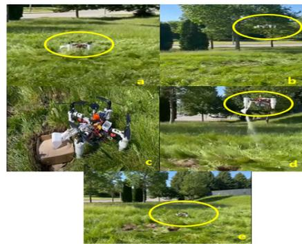
**Figure 5.** The yellow circle highlights the drone in each figure. Drone taking off from the initial point (a), drone en route to be landed landmark (b), drone landmark doing excavation autonomously (c), dumping the excavated soil (d), and the drone arrived back after the excavation operation (e).
