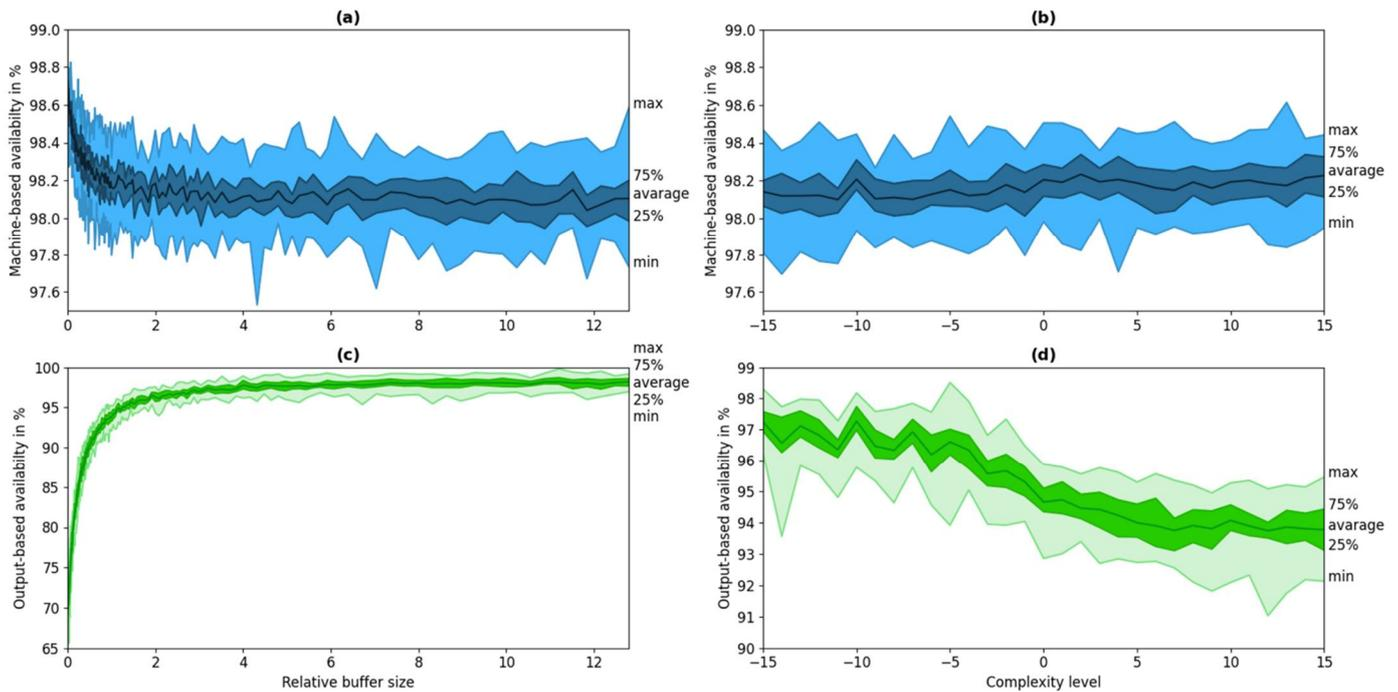
**Figure 2.** (a) Machine-based availability and (c) output-based availability over relative buffer size for complexity level 0; (b) Machine-based availability and (d) output-based availability over complexity for relative buffer size 1.
