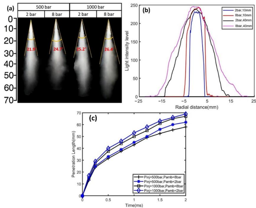
**Figure 4.** (a) Experimental images of diesel spray showing PL and SCA for two different injection and ambient pressures. (b) Light intensity levels with regard to radial distance for 2 axial locations and ambient pressures for 1000 bar injection pressure. (c) PL for diesel spray against varying injection and ambient pressures.
