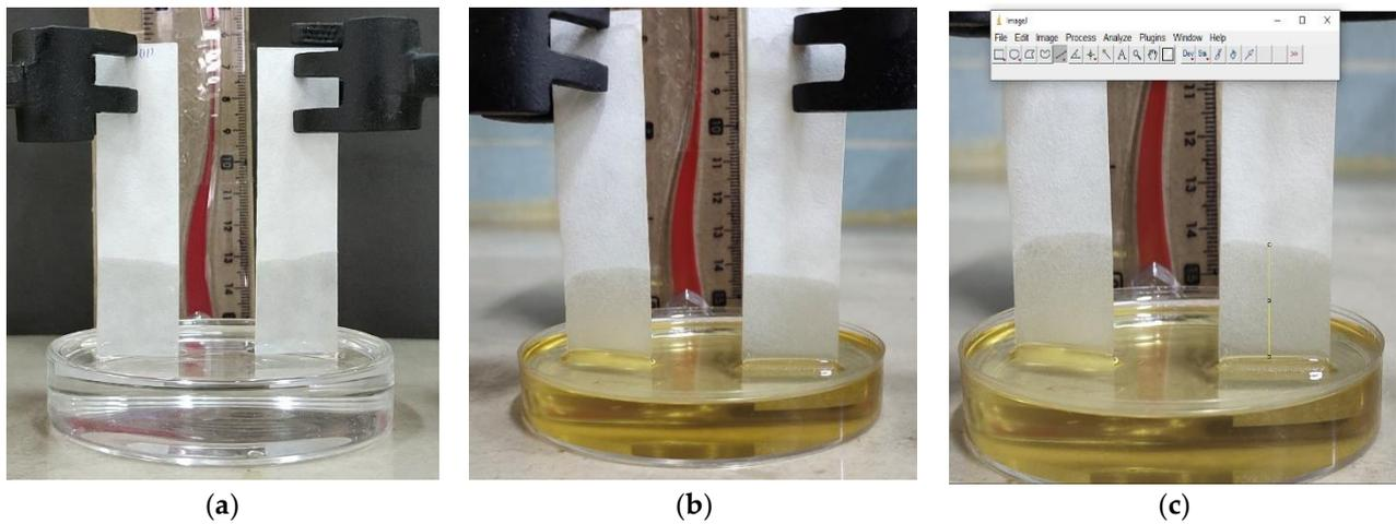
**Figure 2.** Image during experiment: (a) Water flow untreated strip; (b) flow of castor oil in 30% sugar concentration strip; (c) penetration length measured with Image J software (1.48 v).
