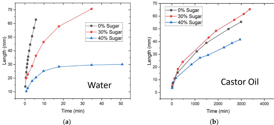
**Figure 3.** Length–time curve: (a) Flow of water in sugar delay zone of different concentrations; (b) flow of castor oil in sugar delay zone of different concentrations.
