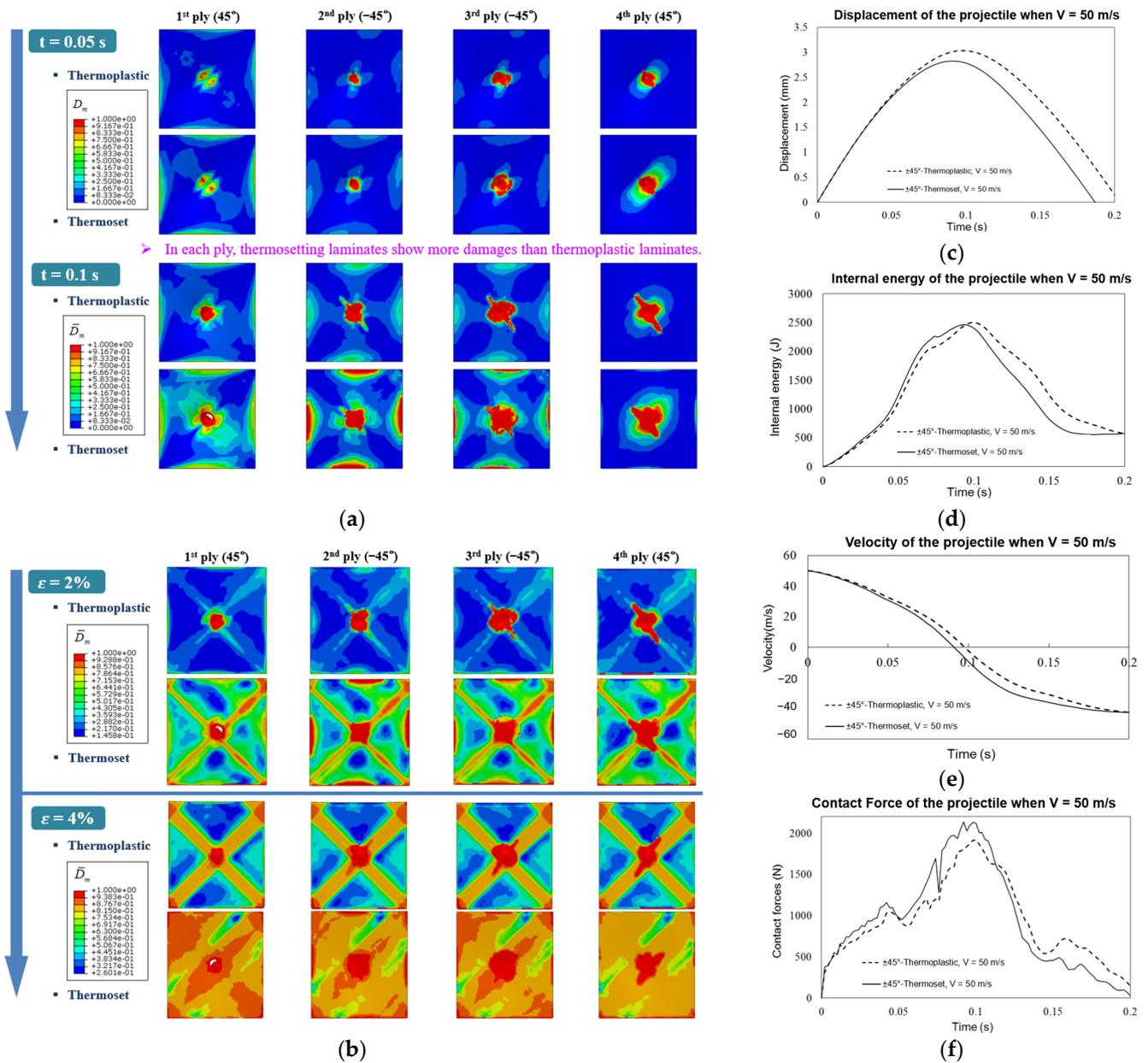
**Figure 2.** (a) Damage contours for Impact; (b) damage contours for CAI; (c) Displacement vs. time graph; (d) internal energy vs. time graph; (e) velocity vs. time graph (f) contact force vs. time graph for BX 45 composite laminates.
