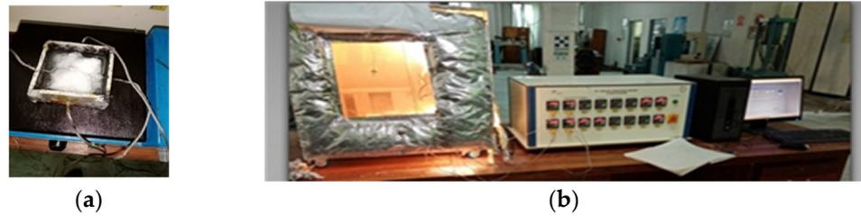
**Figure 2.** (a) Hot-plate heater melts paraffin wax; (b) data logger with a computer system records the temperature of paraffin wax and samples during heating and cooling.
