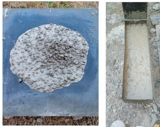
Figure 3. Slump test (left) and L-box test (right).
