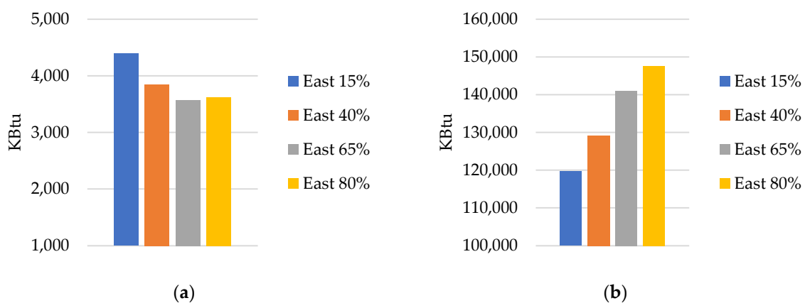
Figure 5. Space (a) heating and (b) cooling consumption in east facing orientation.
