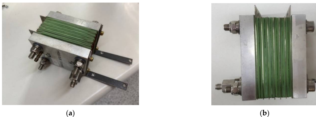
Figure 1. Installed PEM electrolyzer. (a) Overview of the geometry. (b) Detailed view of the structure: cathode, membrane and anode.
