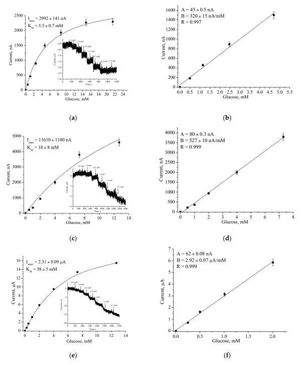
**Figure 3.** Amperometric characteristics of the GO/PO/GE (**a**,**b**), GO/nCuCe/GE (**c**,**d**) and GO/nCuCe/npAu/GE (**e**,**f**): (**a**,**c**,**e**) chronoamperogramms (inserted) and dependences of amperometric signal on concentration of glucose; (**b**,**d**,**f**) calibration graphs for glucose determination. Conditions: working potential –50 mV vs. Ag/AgCl/3 M KCl in 50 mM PB, pH 6.0. The sensing layers contain 0.01 U of PO/PO-like activity and 0.01 U of GO.
