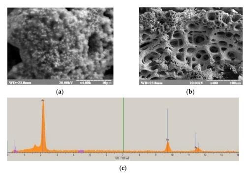
Figure 2. Characteristics of the npAu SEM images (a,b); X-ray spectral microanalysis (c).
