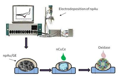
Figure 1. Scheme of electrode modification.
