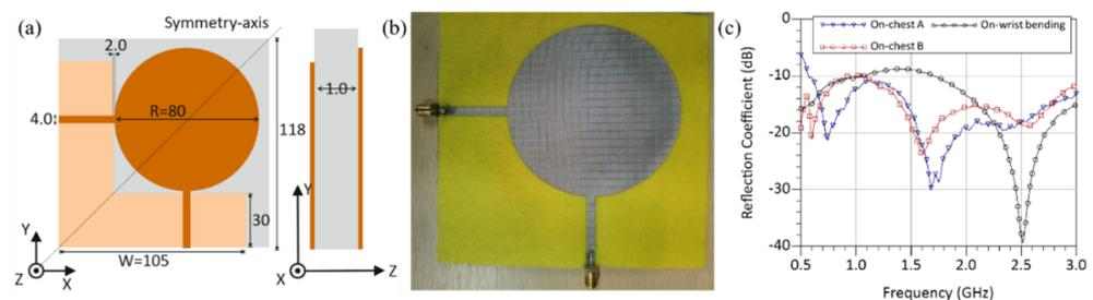
**Figure 1.** The proposed e-textile sensing antenna: (a) layout and dimensions (in mm); (b) photograph of the fabricated prototype; (c) measured reflection coefficient of the antenna on different body parts showing a matched impedance.
