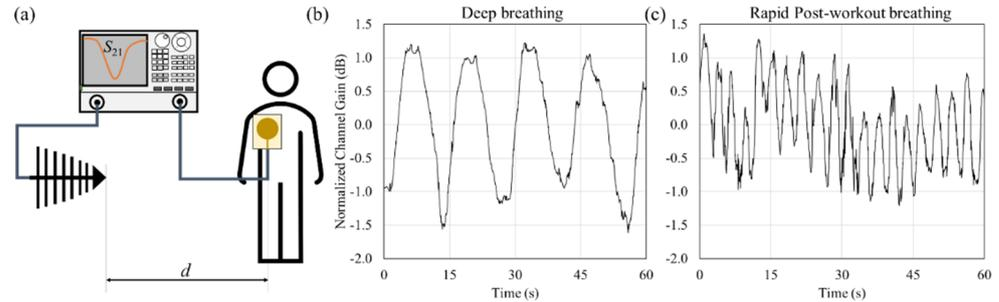
**Figure 2.** Antenna gain measurements showing the breathing patterns: (a) measurement setup; (b) measured channel gain during deep breathing; (c) measured channel gain during rapid breathing.
