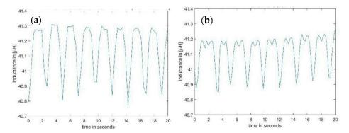
**Figure 4.** Result of a dynamic measurement using the phantom chest (**a**) using the readout circuit given in Figure 3 and converting the frequency back to inductance changes and (**b**) using the precision impedance amplifier (Wayne–Kerr).
