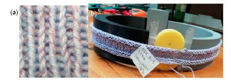
**Figure 1.** (a) Thin insulated metal wire integrated in the knit stitches that form the 3D helical coil. (b) The chest phantom holding a test coil. The oval disk is connected to a small motor to rotate it around its axis over programmed angles and with a given speed.
