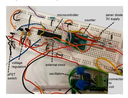
**Figure 3.** The circuit of Figure 3 implemented on a breadboard.
