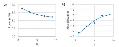
**Figure 5.** (a) Power consumed by the circuit (excluding the microprocessor) as a function of the number of turns N. (b) The variation in the frequency as a function of variation of circumference l. The knit is a 1/1 rib knit in cotton. The chest phantom of Figure 2 is used for static measurements using the thin plastic sliders to increase circumference.
