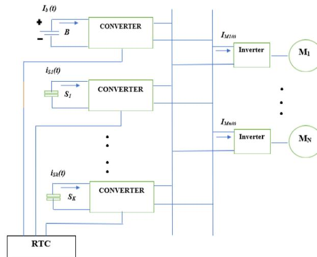
Figure 1. Block diagram of considered HESS Topology.
