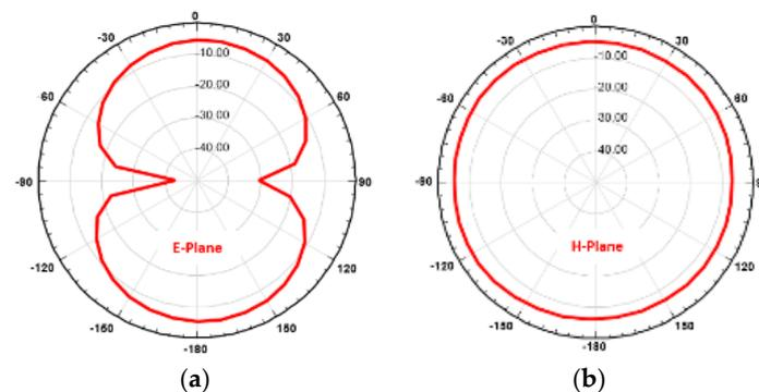
**Figure 4.** Radiation pattern of the proposed antenna: (a) E plane and (b) H plane.
