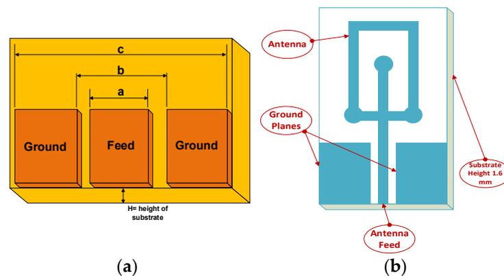
**Figure 1.** (a) Feed line structure; (b) the complete antenna design with major components.
