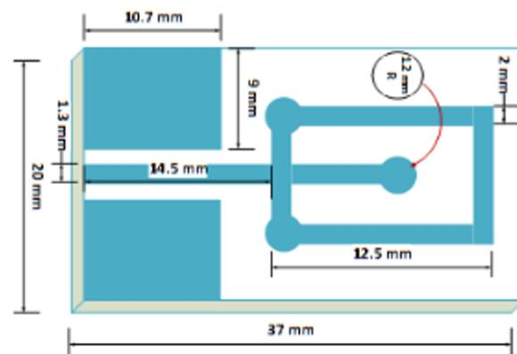
**Figure 2.** The geometry of the proposed antenna.
