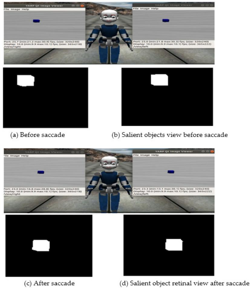
**Figure 1.** Humanoid robot iCub simulator’s saccadic eye movements with reference to learnt motor commands. (a) represents the object location at retina of both eyes before saccadic movements; (b) shows object retinal view of both eyes before saccadic movements; (c) shows saccadic movements of eyes by learnt motor. (d) shows saccadic retinal view of eyes by learnt motor after saccade.
