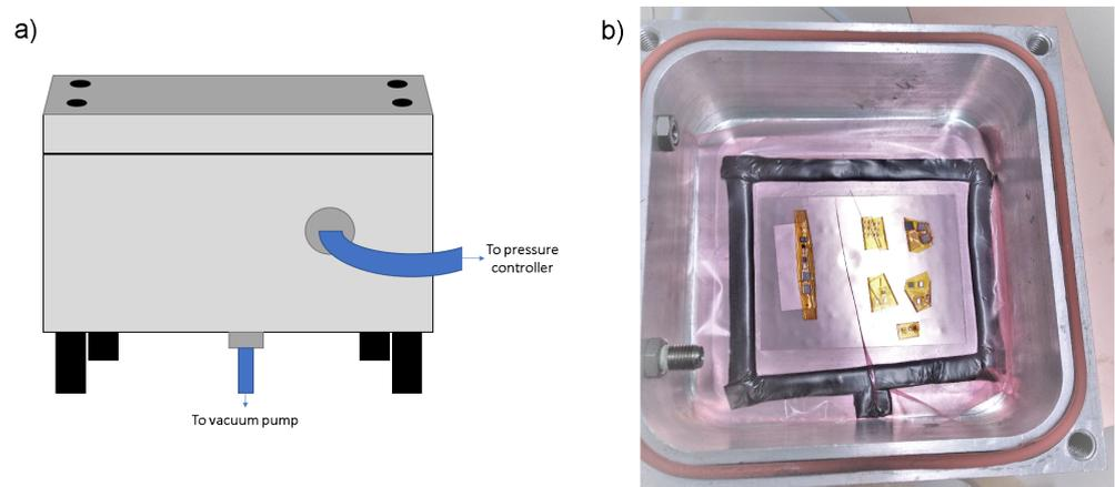
**Figure 3.** Steel box with gasket, inserted component test-plate and applied vacuum bagging film before insertion into the oven. (a) Schematic view of the pressure chamber. (b) Photography of the prepared chamber.
