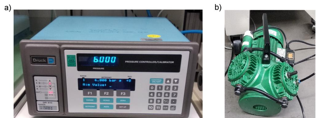
**Figure 2.** Pressure control equipment. (a) Pressure controller. (b) Vacuum pump.
