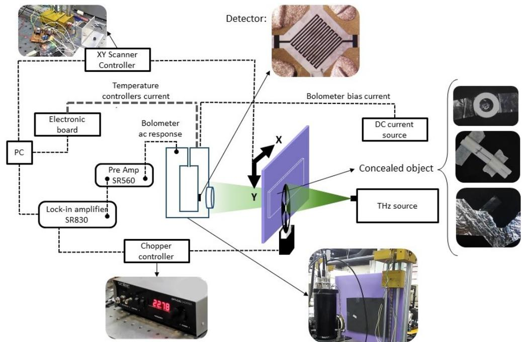
Figure 1. Schematic of the imaging setup.
