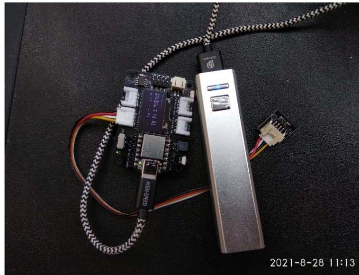
**Figure 4.** Temperature measurement setup with the conventional air temperature sensors AHT20 and BMP280 on the same board.
