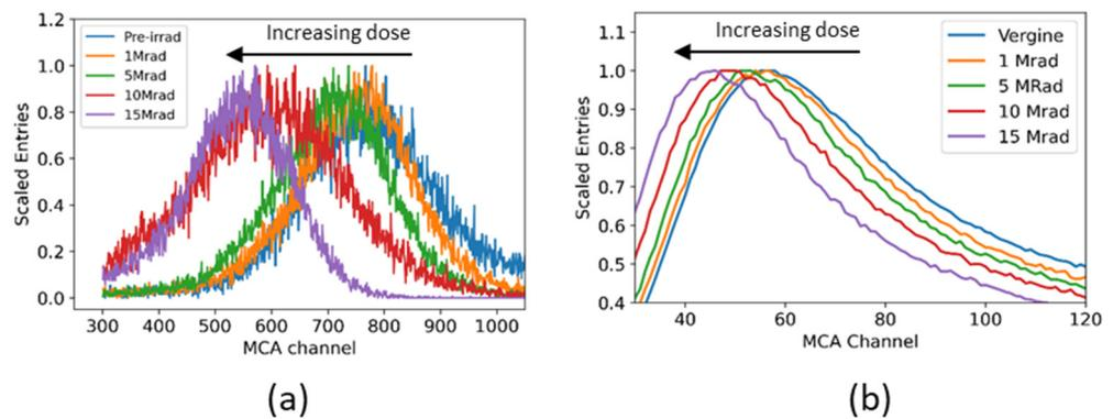
**Figure 3.** Light yield spectra of proton irradiated thin-film PEN scintillators excited by (a) alpha particles from a <sup>241</sup>Am source and (b) electrons from a <sup>137</sup>Cs source.
