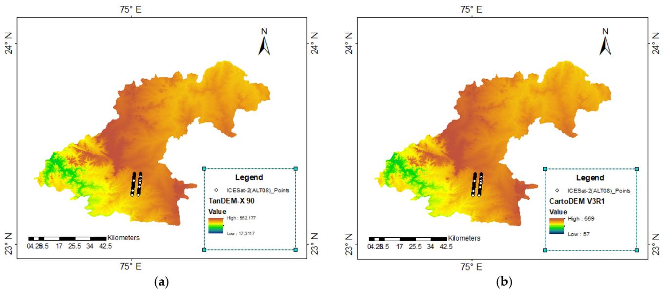
**Figure 3.** (a) ICESat-2 (ALT08) points superimposed on TanDEM-X 90; (b) ICESat-2 (ALT08) points superimposed on CartoDEM V3 R1.
