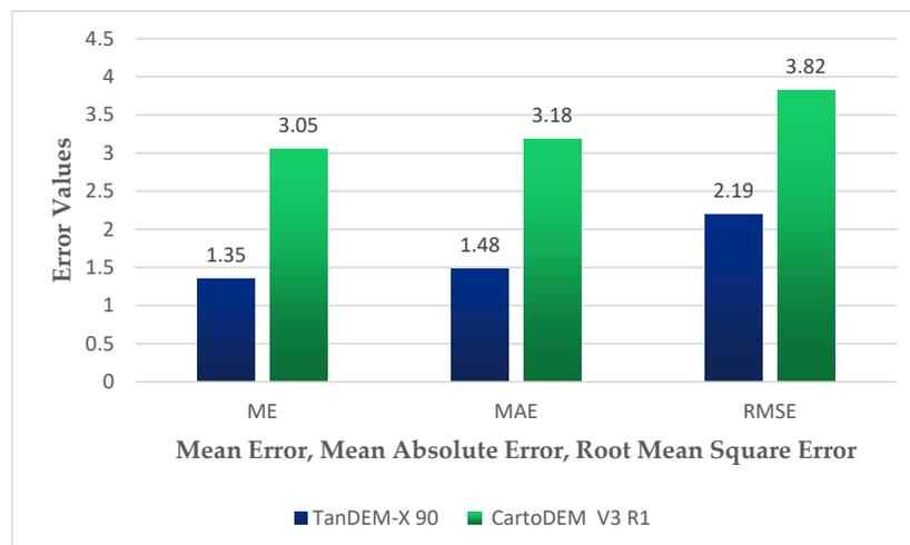
**Figure 4.** Plot of ME, MAE, and RMSE for TanDEM-X 90 and CartoDEM V3 R1 with ICESat-2 elevation data as a reference.
